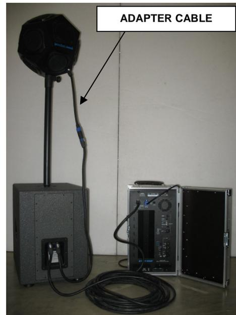
Figure 7: Connections to amplify only JA12. PRESET: "JA12"
