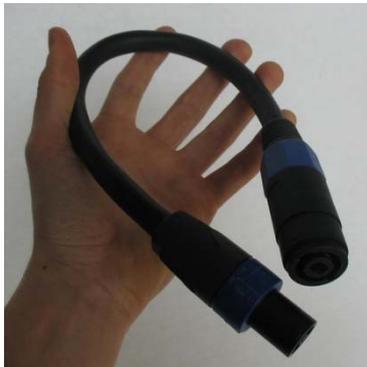
Figure 6: Adapter cable for JA12
