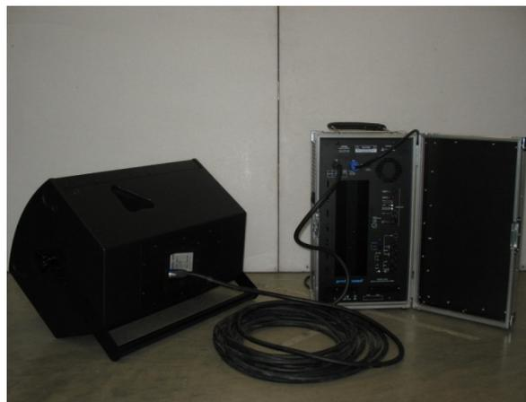
Figure 9: Connections for JA4012 directional source. PRESET: "JA40"
