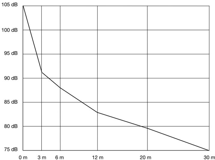
The above diagrams clearly illustrate the significant reduction in sound level that can be achieved outside the floor by using the AS120 Crossfire system instead of a traditional speaker.
