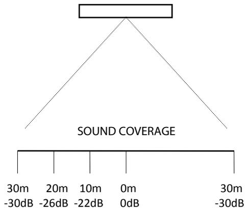
With the revolutionary AS120 Crossfire system, the drop in sound level at 10 metres from the centre of the floor is already **-22 dB** and at 30 metres can be as much as **-30 dB**.
