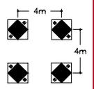
B) Spectrum measurement of the sound level produced at 1.5 metres from the ground by four AS120 speakers mounted in operating position, 4 metres from each other, at a height of 3.5 metres from the reflecting floor, pointing downwards.
