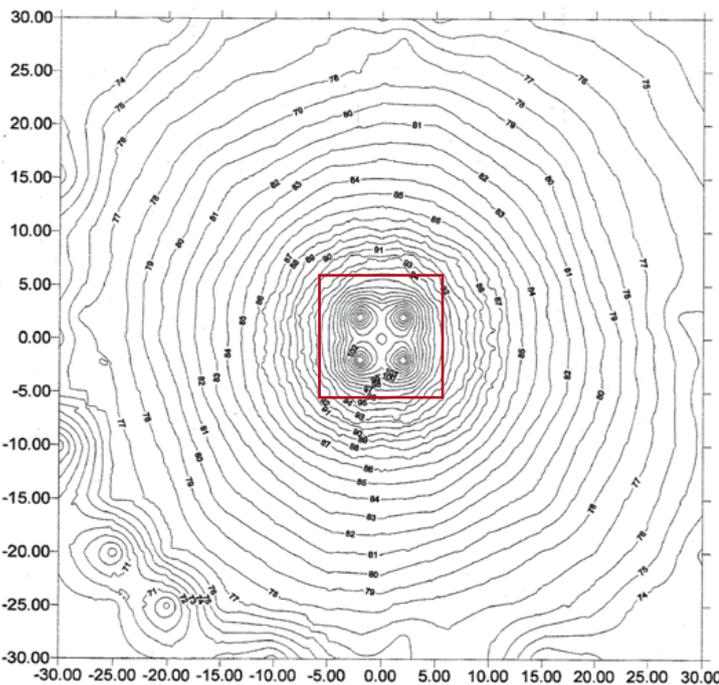
We notice that four speakers produce a much more homogeneous sound distribution across the floor. Placing the speakers at 6 metres from each other reduces the difference from the centre to the edge of the floor from 15 dB to just 7 dB.
