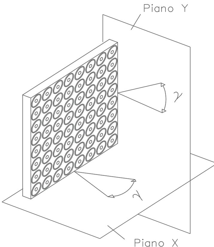
Dwg 3. With Peecker Sound double array the sound beam gets thinner in both directions
