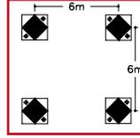
C) Spectrum measurement of the sound level produced at 1.5 metres from the ground by four AS120 speakers mounted in operating position, 6 metres from each other, at a height of 3.5 metres from the reflecting floor, pointing downwards.
