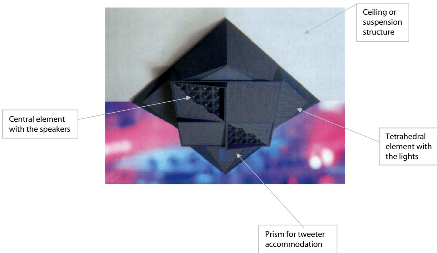
Figure 6. AS120 Crossfire acoustic loudspeaker system
