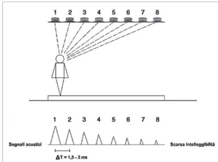
Figure 1. Layout scheme of forward firing loudspeakers
