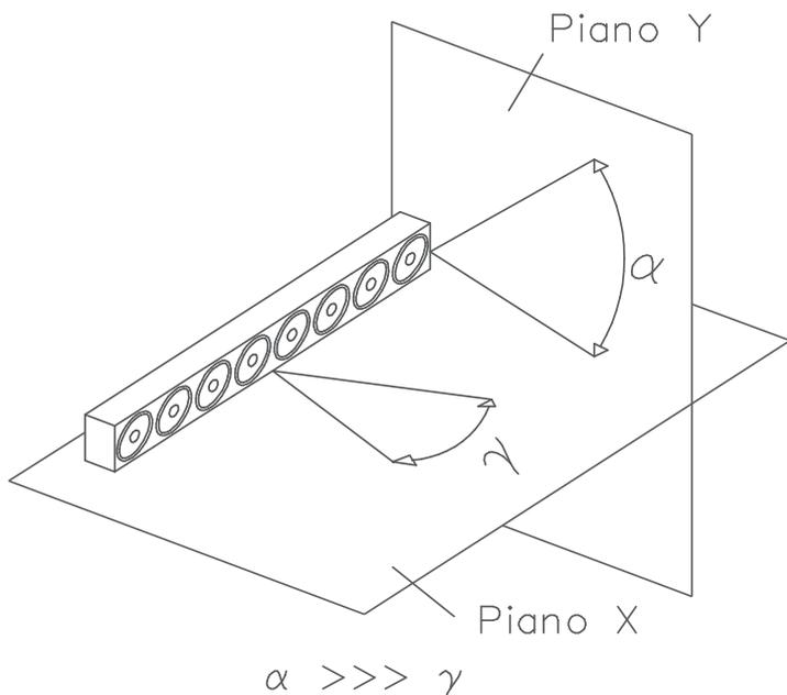
Dwg 2. With a single line array (positioned on plane X) the sound beam is very narrow in the horizontal direction, but it remains very wide in the vertical one
