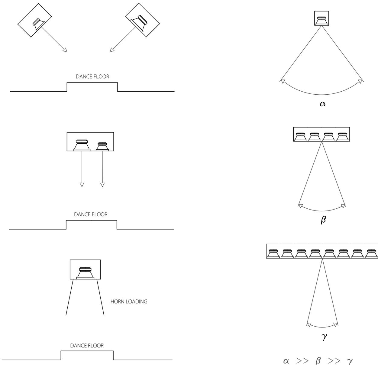
Dwg 1. Dispersion angle differences between standard horn-loaded speakers and line arrays (4 and 8 elements)
