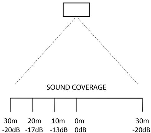
With a standard loudspeaker system, the sound level at 10 metres from the centre of the floor drops by just **-13 dB** and at 30 metres by **-20 dB**.
